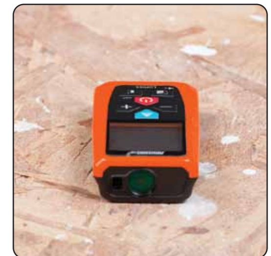
Cal3: Rotate 180°, LCD towards you.
