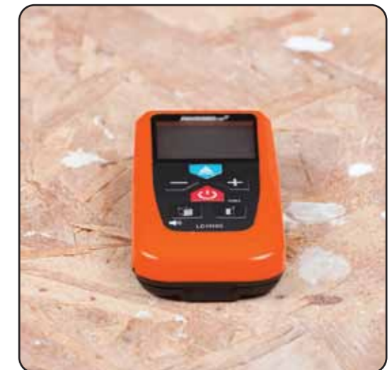
Cal2: Lay down flat, LCD away from you.
